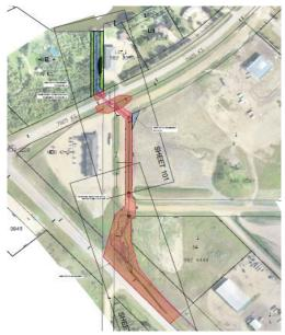
improvements in the south industrial subdivision consisting of the installation of two new culverts (one at the bend of 43 avenue & one at the bend of 49th street service road heading south), decommissioning of existing culverts in the area, with a new culvert system under highway 881 tying into the construction of a new drainage ditch on the west side of highway 881 going down to Hardisty Lake.
